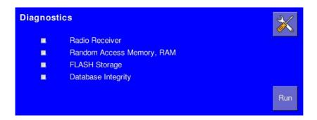
Radio Receiver: If OK, displays the average signal strength in dBm.
