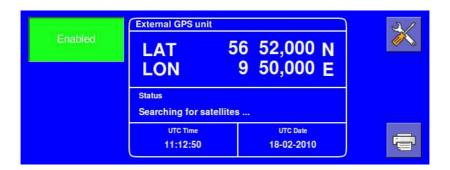
If a printer is connected you can press to print a position label with UTC Time and Date. These labels are useful when you write positions in the logbook or in case of an emergency.
