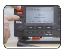
Lift the lid to the DISTRESS button and push the button for a minimum of three seconds.
