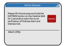
Press the DISTRESS button on the LT-3100S Control Unit to activate the Terminal Test.
