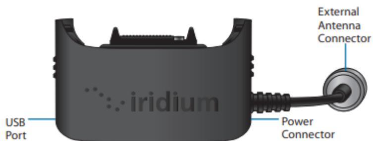
Please note that it is recommended if you are sitting inside using your computer to use the external antenna for a good signal. The antenna must have clear view to the sky.
