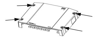
Figure 34: Disassembling - remove cover
