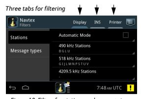
Figure 10: Filters for stations and message types
