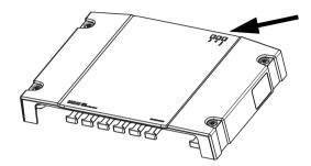
Figure 28: System LEDs
