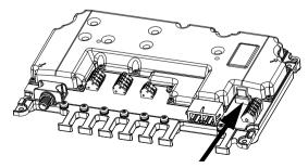
Figure 35: Replace the fuse
