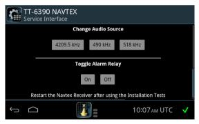
Figure 26: Service Interface, toggle alarm relay
