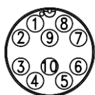
Figure 44: AUX connector (pin out)
