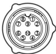
Figure 45: AUX cable (pin out)
