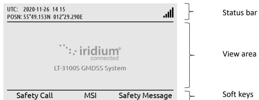
Figure 65: LT-3110S Control Unit (display sections)
