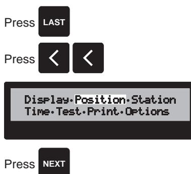
The cursor is now flashing which indicates that an input is expected; this case you have to enter the time when the position was valid. Use the numerical keyboard to enter the time. If you enter an incorrect digit, you can delete the digit by pressing the  $\leftarrow$  key.
