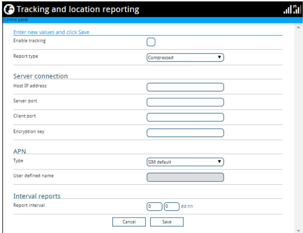
2. To enable tracking of the EXPLORER 540, select **Enable tracking**.
