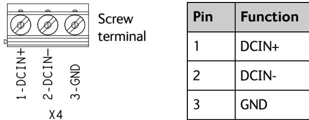
To unscrew and fasten the screws in X4 use a screwdriver (max. 3.5 mm wide). If the DC cable is shielded, connect the shield to pin 3, GND. Otherwise leave GND unconnected.
