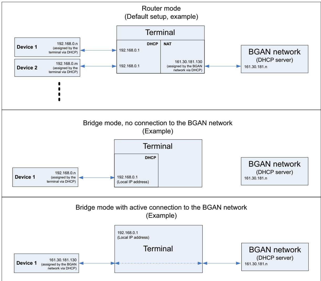
To set up the connection mode of the EXPLORER 540, do as follows:
