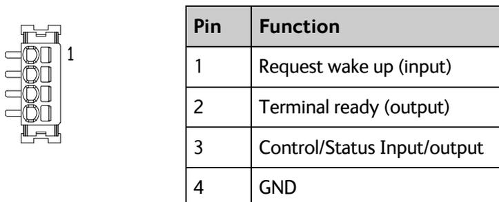
To insert the wires in X5 use a screwdriver (max. 2mm wide) to push each terminal open. For configuration of the I/O pins, see *Power save* on page 88
