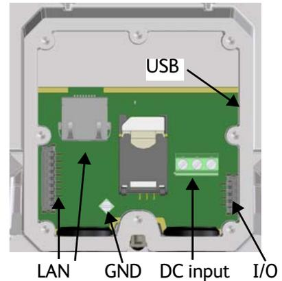
**Note** If you are going to use the optional EXPLORER 540 LTE Modem, connect the modem to the USB connector. For details see the installation guide included with the EXPLORER 540 LTE modem.
