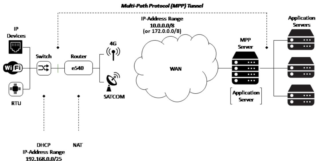
To set up PRISM you must install the PRISM server software from Cobham SATCOM, configure the PRISM server and set up your EXPLORER 540 to communicate with this server.
