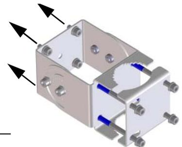
2. Unscrew two of the long screws from the pole mount kit to leave one side open for the pole.
