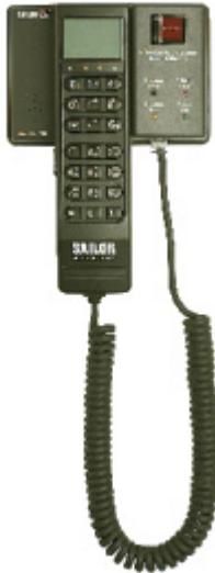
The cradle has a distress button, a stop button and three LEDs. The distress button, which is protected by plastic glass, is used to initiate a distress call. The stop button can be used to abort a distress call. The three LEDs indicate power, distress test and priority calls. For a detailed description of the cradle see the section *Distress Cradle* on page 33.
