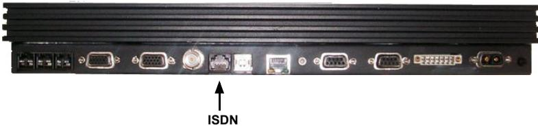
This interface can be used for connection of ISDN equipment – data as well as voice/picture based equipment (phones, modems, terminal adapters, audio codecs, video conferencing equipment, STE secure voice, etc.).
