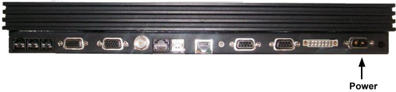
The Power connector must be connected to a 24 V DC floating power supply. For information on how to connect power, see the Installation Manual.
