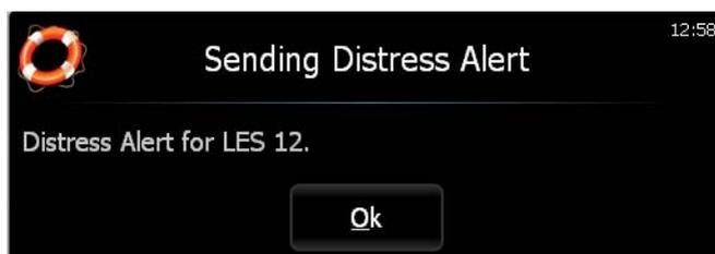
The display also shows when the Distress Alert is acknowledged from the LES. **Write down the LES number** - you must use the same number when you send a Distress message with more information for the MRCC.
