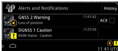
Figure 34: Alerts and notifications from GNSS/DGNSS Receivers
