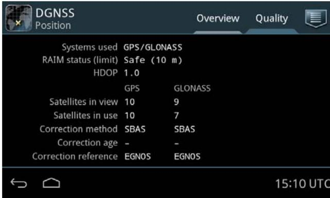
Figure 17: Using SBAS corrections
