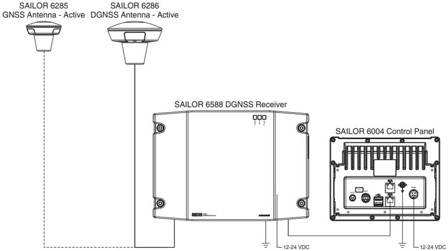
Figure 1: System configuration
